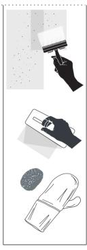
brush and obtain the finished effect either with a sponge float of a woolen glove which is used for decorating. The velatura classic finish made up of **NEO** acrylic paint and Murano Velatura.
